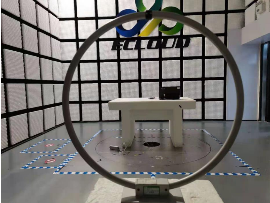
Fig. 1 Radiated emission setup photo(Below 30MHz)
