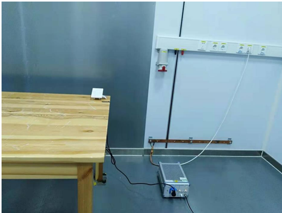
Fig. 4 Power line conducted emission setup photo
