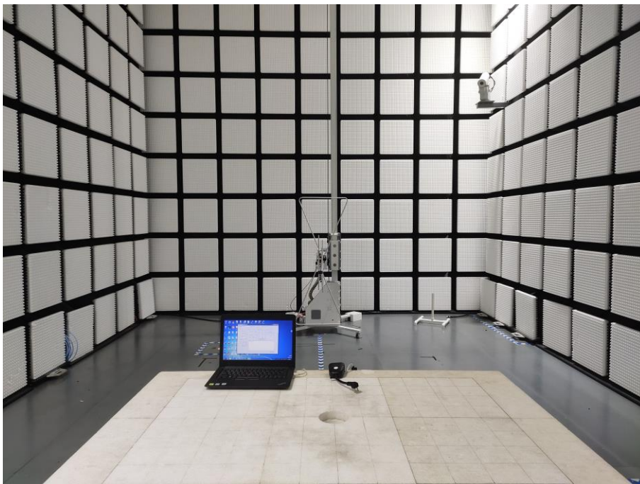
Fig. 2 Radiated emission setup photo(30MHz-1GHz)
