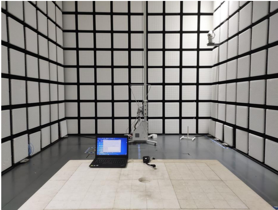
Fig. 1 Radiated emission setup photo(30MHz-1GHz)
