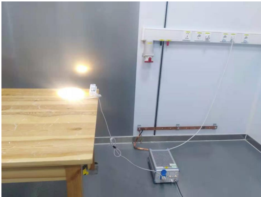
Fig. 4 Power line conducted emission setup photo
