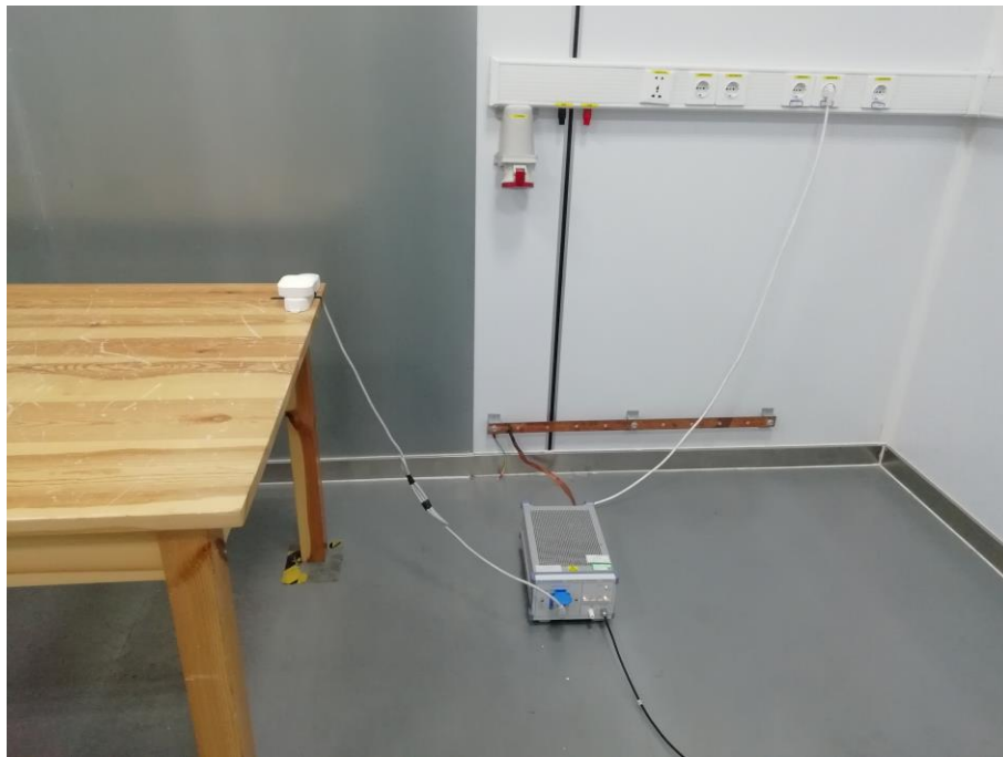
Fig. 4 Power line conducted emission setup photo
