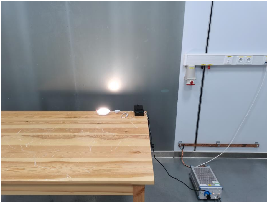
Fig. 3 Power line conducted emission setup photo
