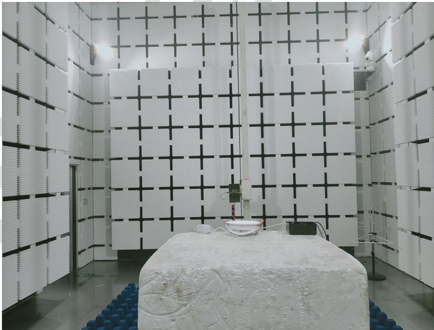
Conducted Emissions at AC Power Line (150kHz-30MHz)
