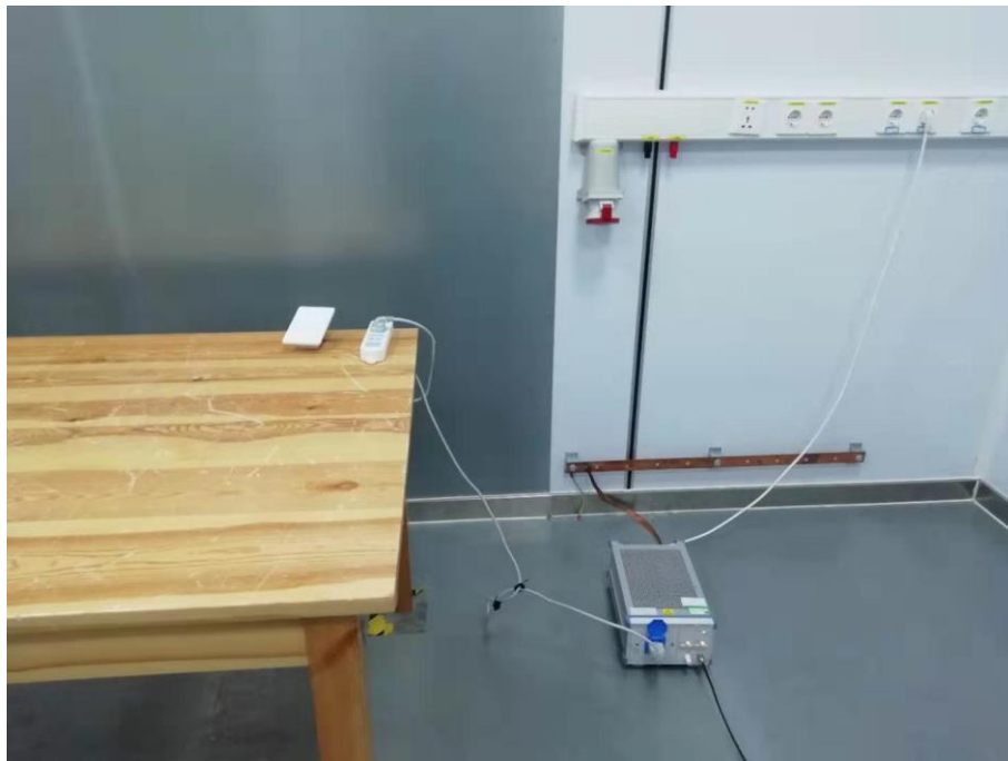
Fig. 4 Power line conducted emission setup photo
