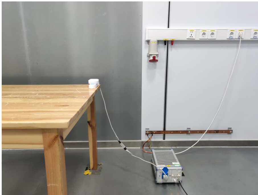
Fig. 4 Power line conducted emission setup photo
