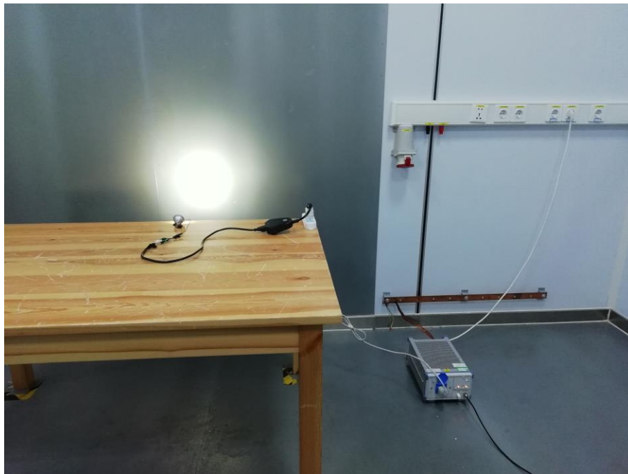
Fig. 4 Power line conducted emission setup photo
