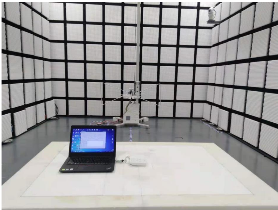
Fig. 2 Radiated emission setup photo(30MHz-1GHz)
