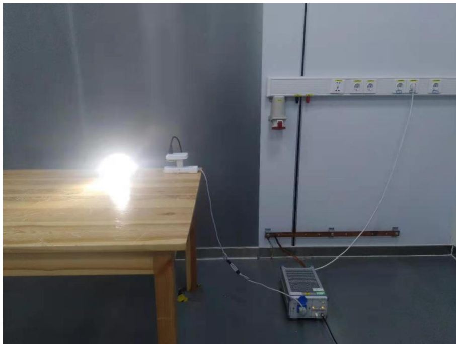
Fig. 4 Power line conducted emission setup photo
