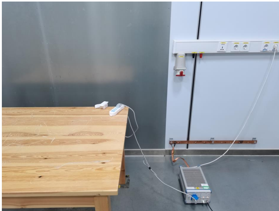
Fig. 4 Power line conducted emission setup photo
