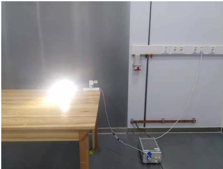
Fig. 4 Power line conducted emission setup photo
