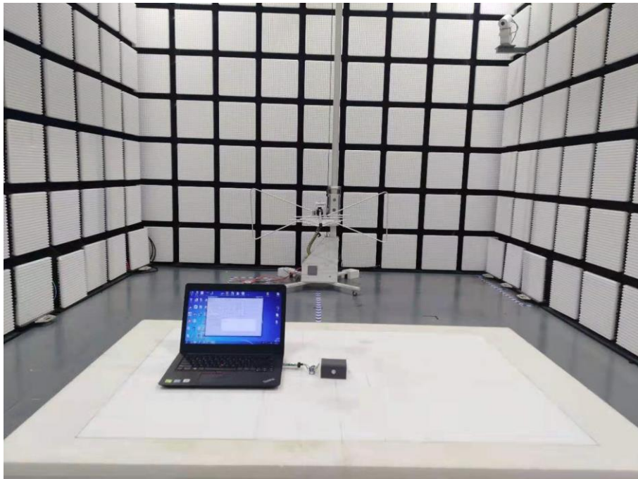
Fig. 2 Radiated emission setup photo(30MHz-1GHz)
