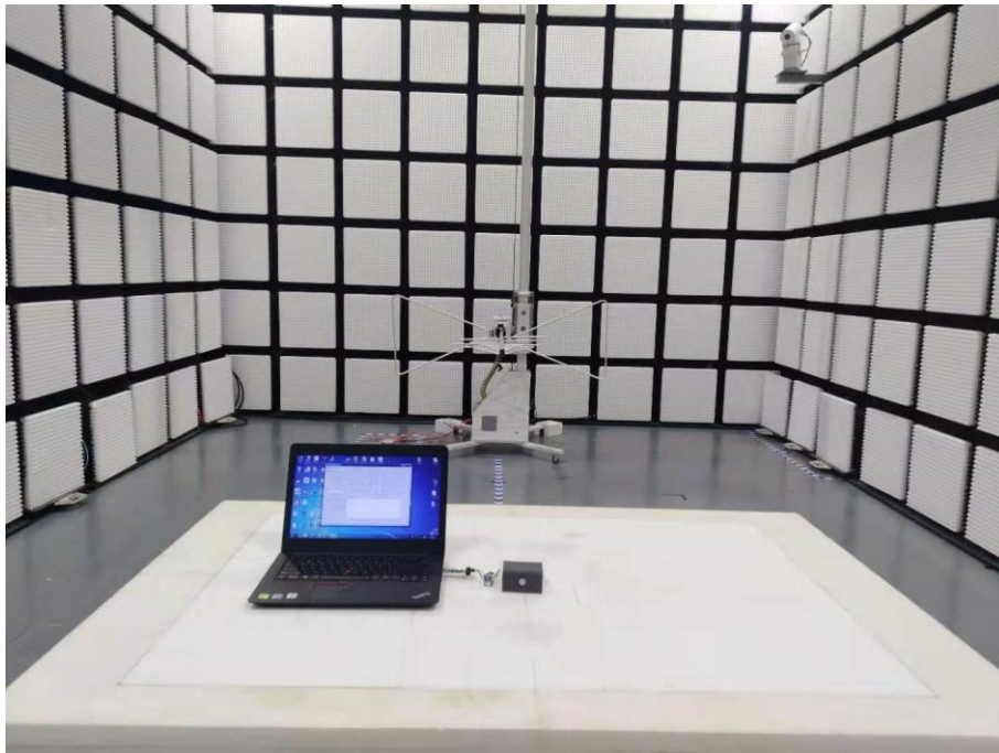
Fig. 2 Radiated emission setup photo(30MHz-1GHz)
