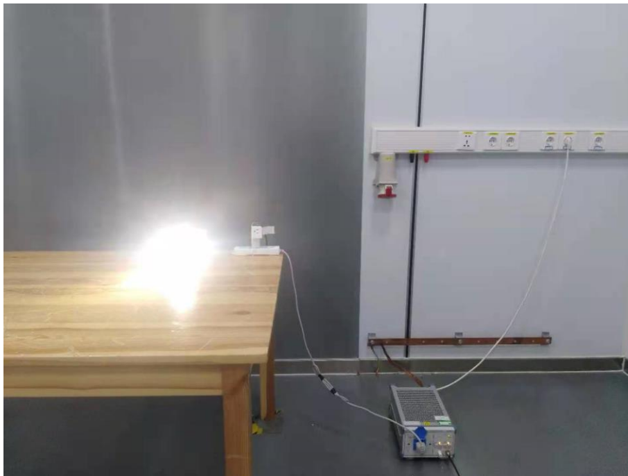
Fig. 4 Power line conducted emission setup photo
