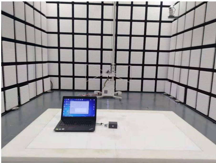
Fig. 2 Radiated emission setup photo(30MHz-1GHz)
