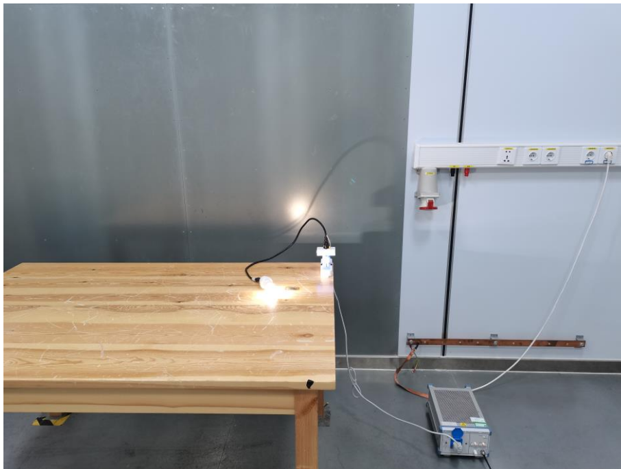
Fig. 4 Power line conducted emission setup photo
