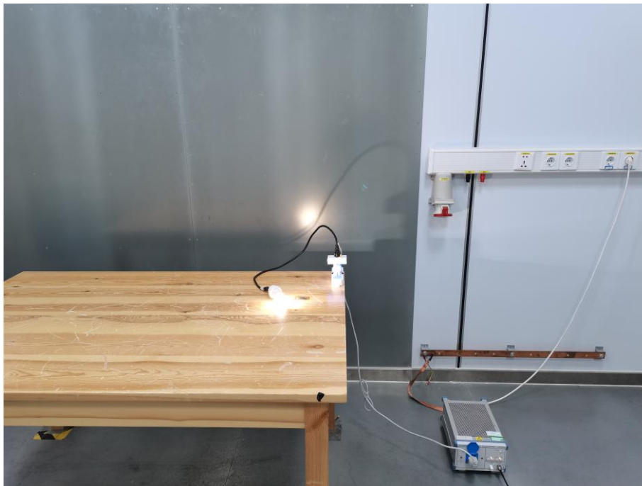
Fig. 4 Power line conducted emission setup photo
