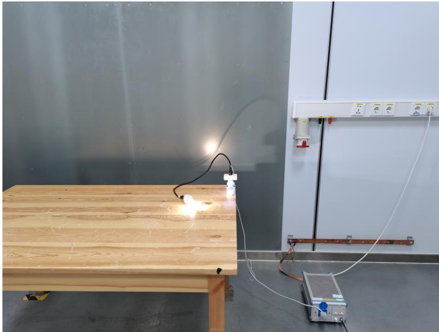
Fig. 4 Power line conducted emission setup photo
