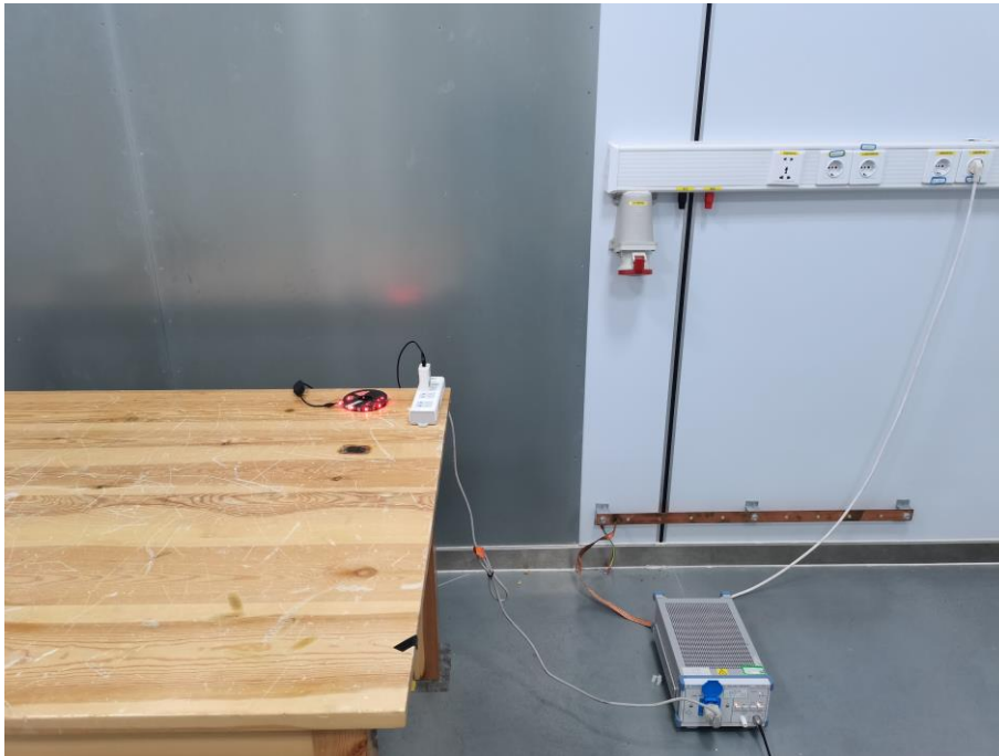
Fig. 4 Power line conducted emission setup photo
