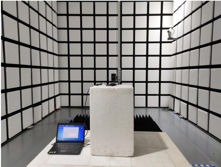
Fig. 3 Radiated emission setup photo(Above 1GHz)
