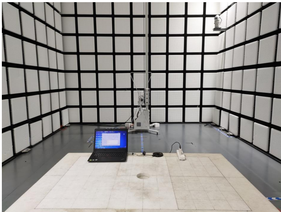
Fig. 2 Radiated emission setup photo(30MHz-1GHz)
