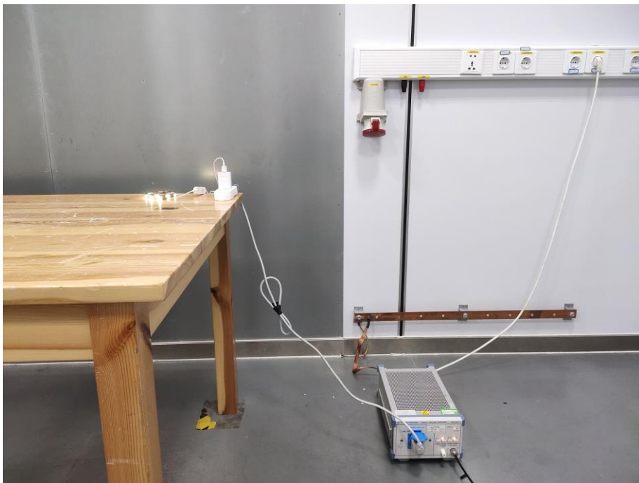
Fig. 4 Power line conducted emission setup photo
