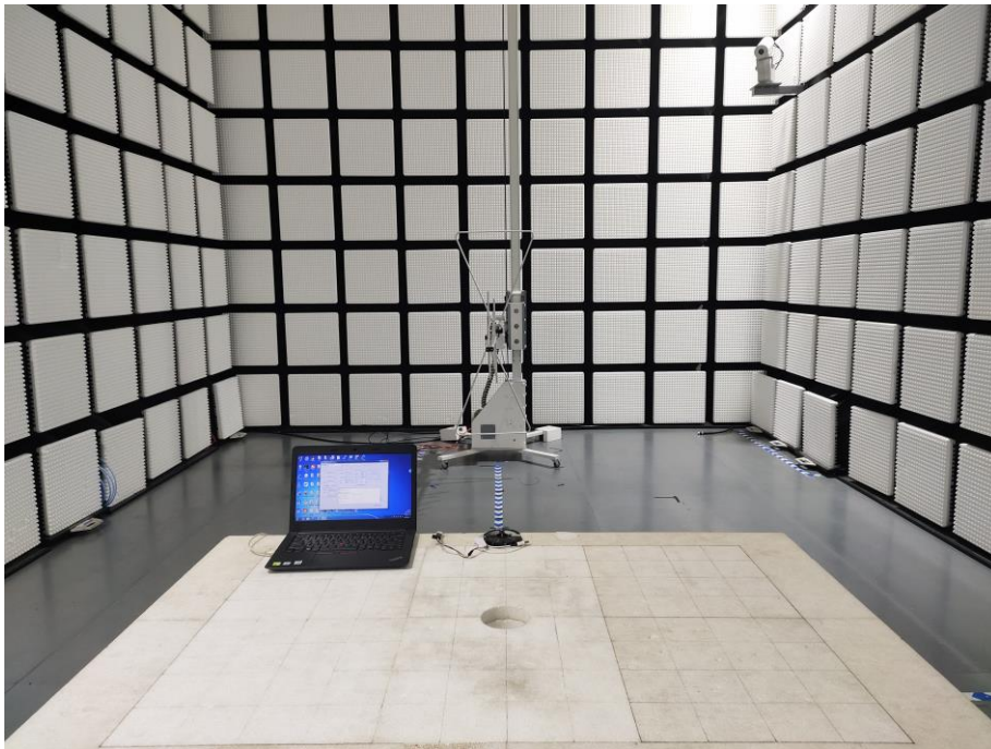
Fig. 2 Radiated emission setup photo(30MHz-1GHz)
