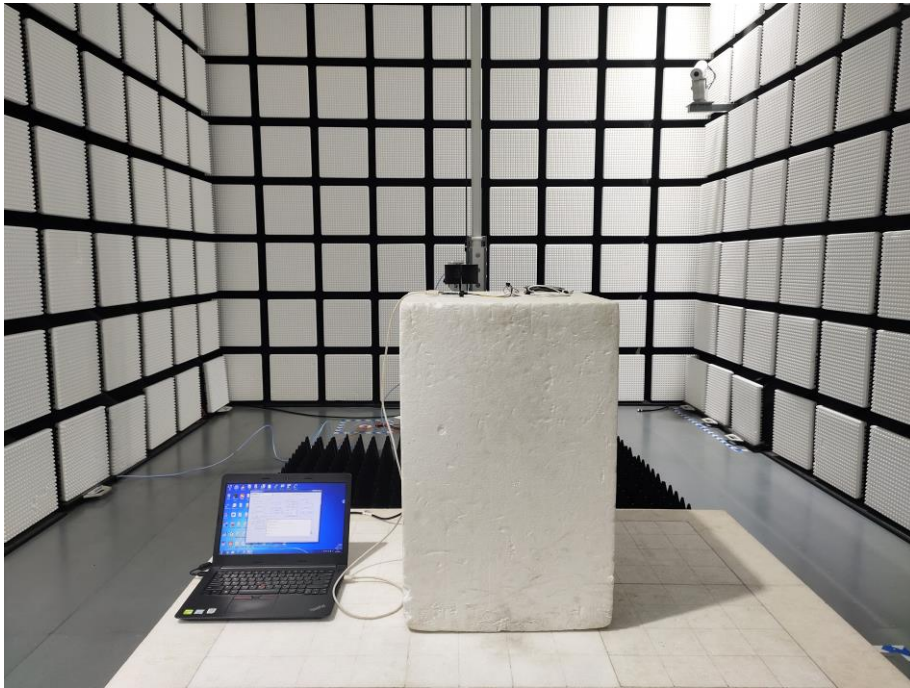
Fig. 3 Radiated emission setup photo(Above 1GHz)
