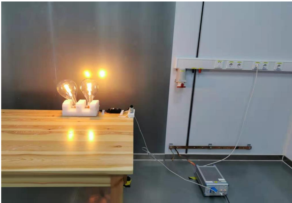
Fig.4 Power line conducted emission setup photo
