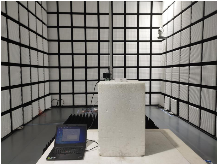
Fig. 3 Radiated emission setup photo(Above 1GHz)
