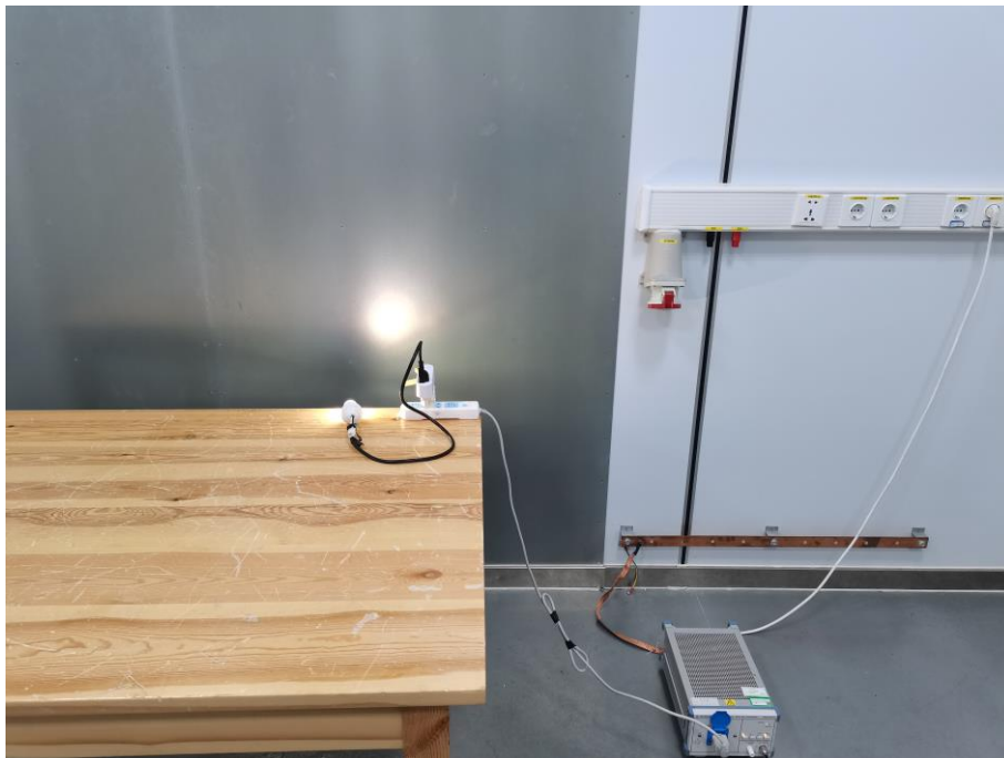
Fig. 4 Power line conducted emission setup photo
