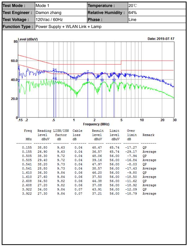
Result Level= Reading Level + LISN Factor + Cable Loss
