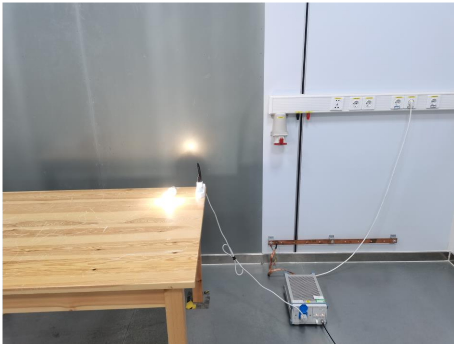
Fig. 4 Power line conducted emission setup photo
