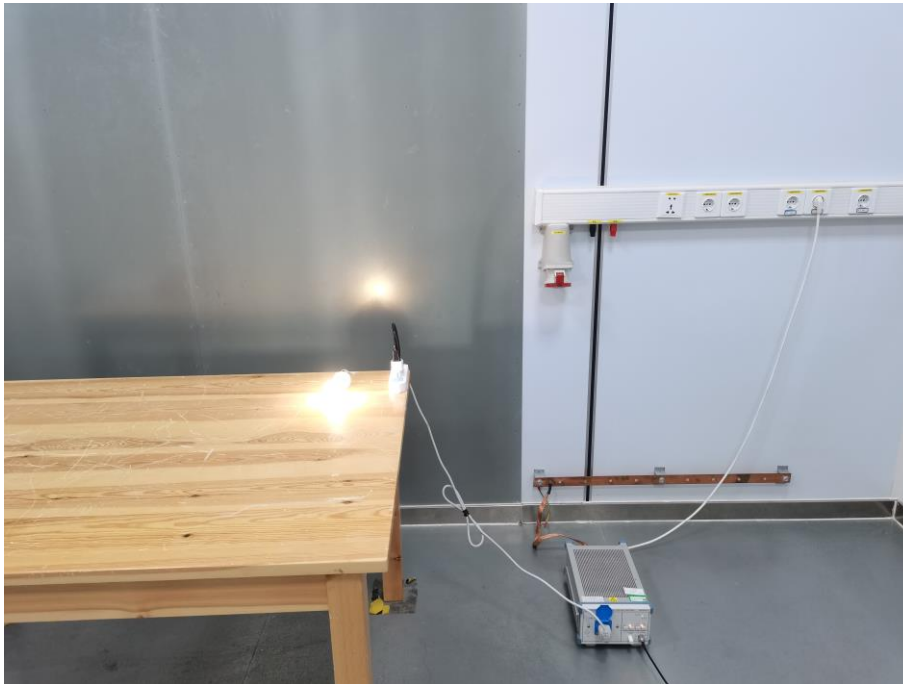
Fig. 4 Power line conducted emission setup photo
