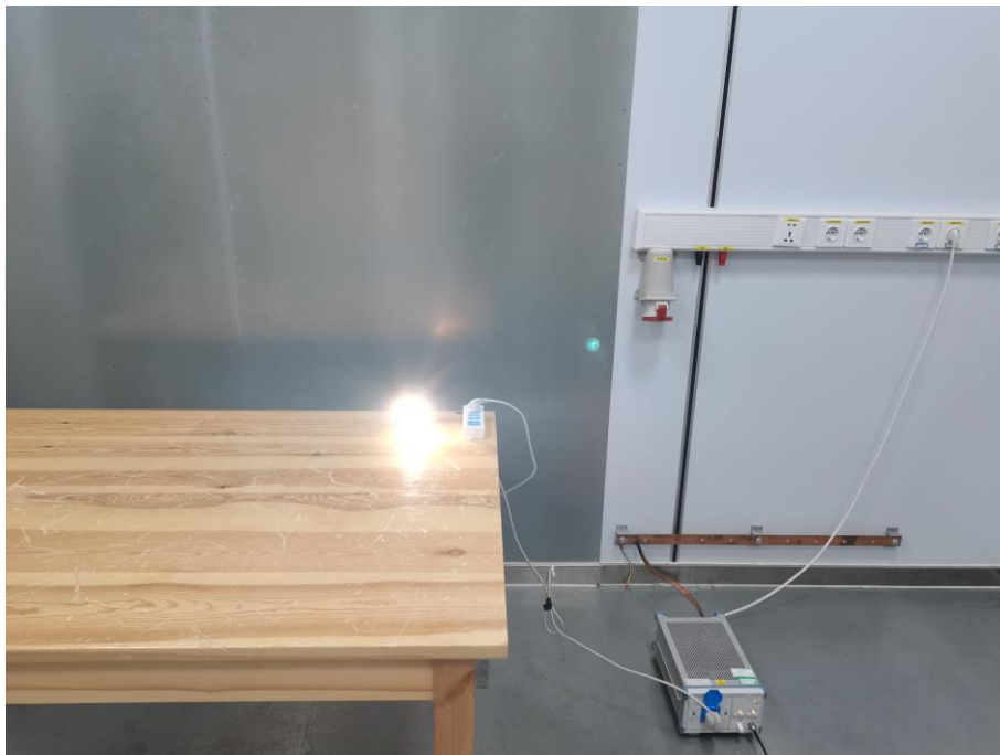
Fig. 4 Power line conducted emission setup photo
