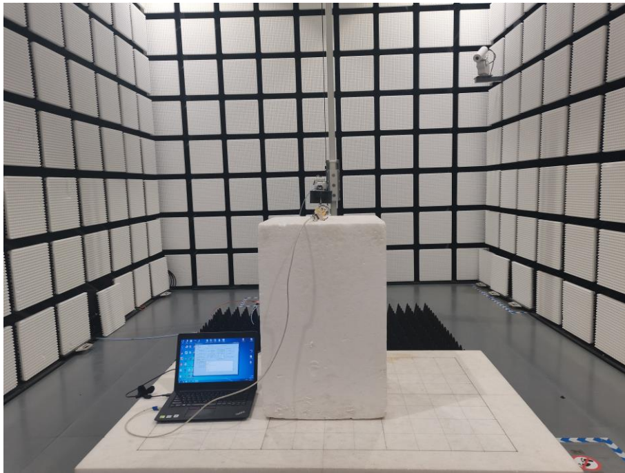
Fig. 3 Radiated emission setup photo(Above 1GHz)
