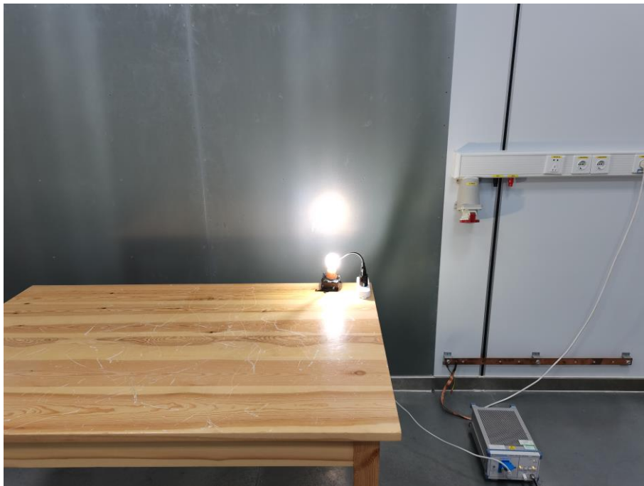
Fig. 4 Power line conducted emission setup photo
