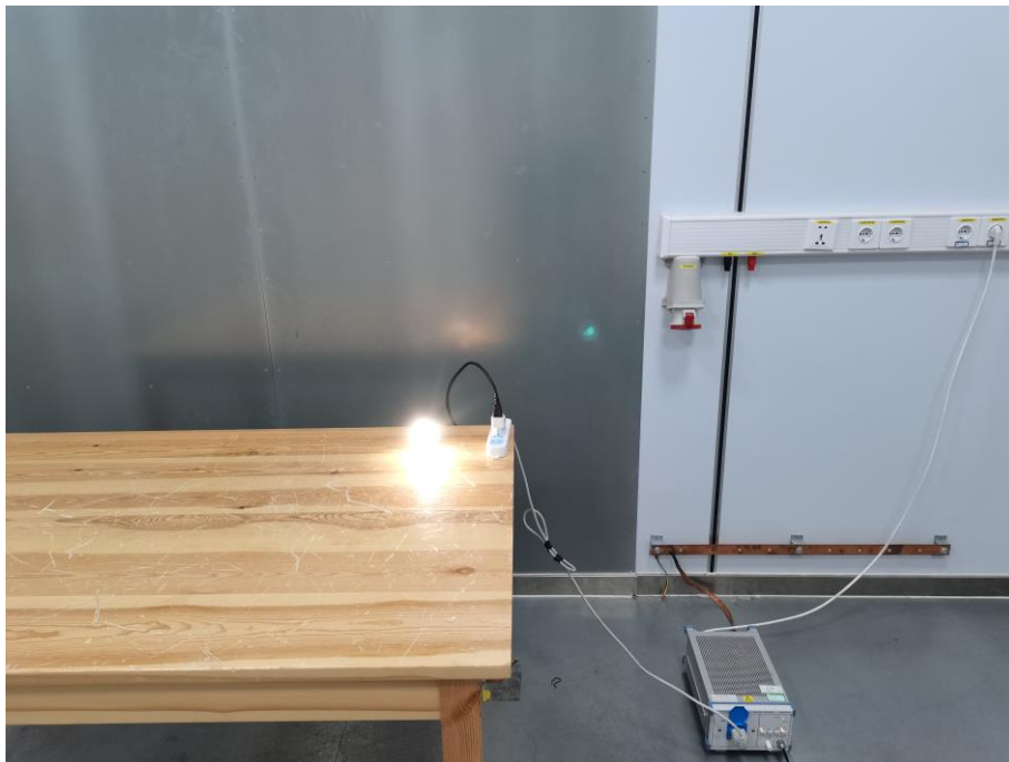
Fig. 4 Power line conducted emission setup photo
