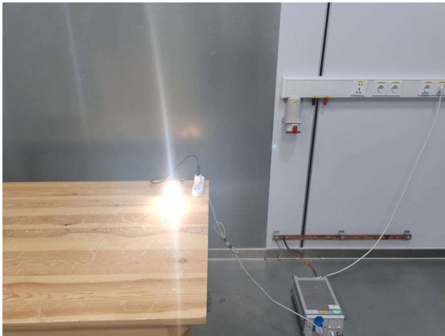
Fig. 4 Power line conducted emission setup photo
