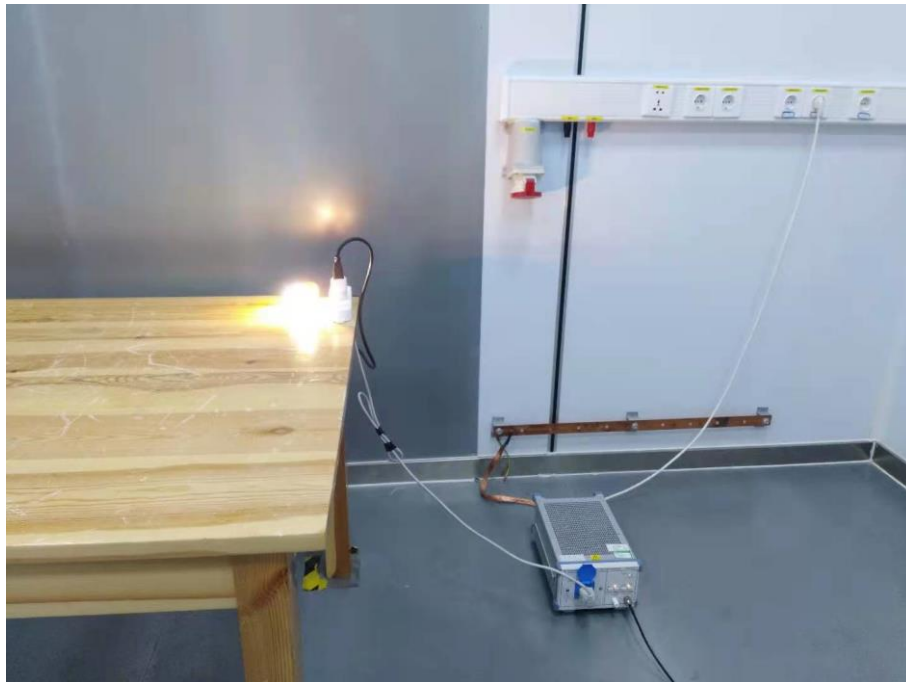
Fig. 4 Power line conducted emission setup photo
