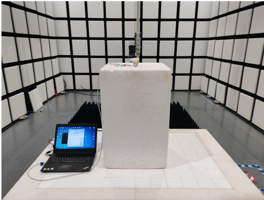
Fig. 3 Radiated emission setup photo(Above 1GHz)
