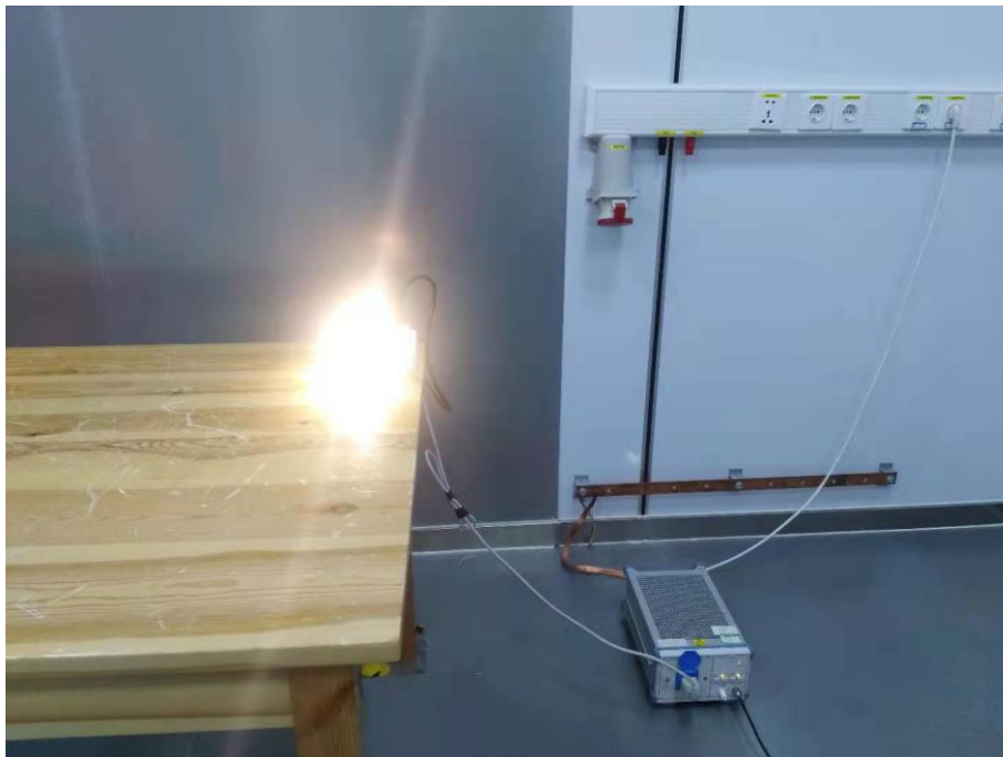
Fig. 4 Power line conducted emission setup photo
