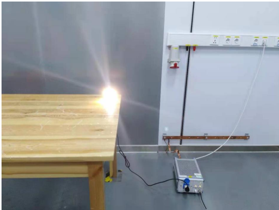
Fig. 4 Power line conducted emission setup photo
