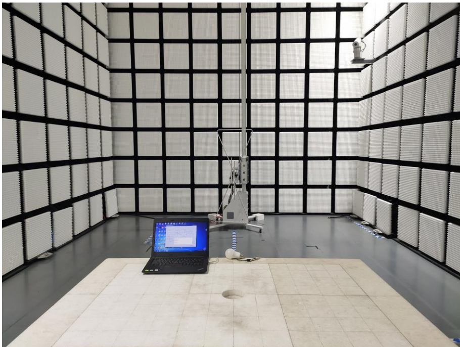
Fig. 2 Radiated emission setup photo(30MHz-1GHz)
