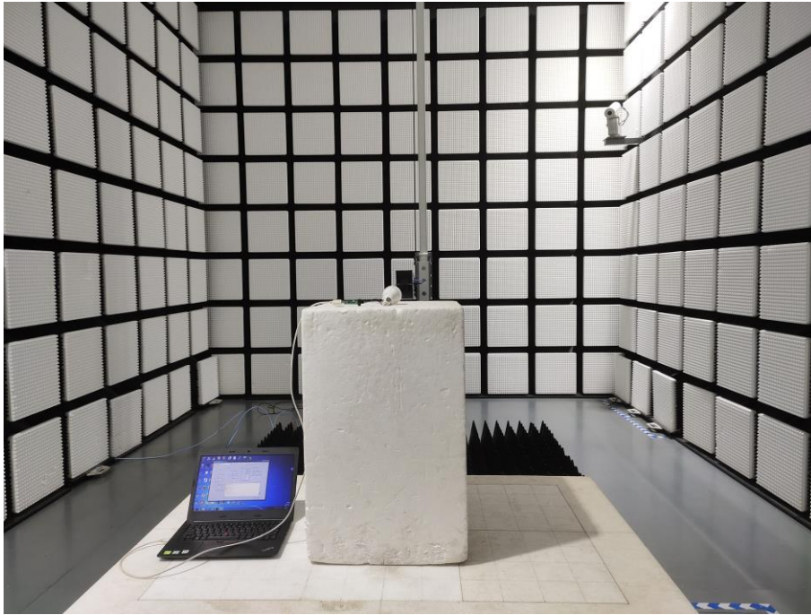
Fig. 3 Radiated emission setup photo(Above 1GHz)
