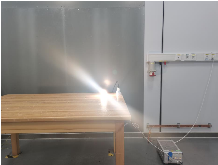
Fig. 4 Power line conducted emission setup photo
