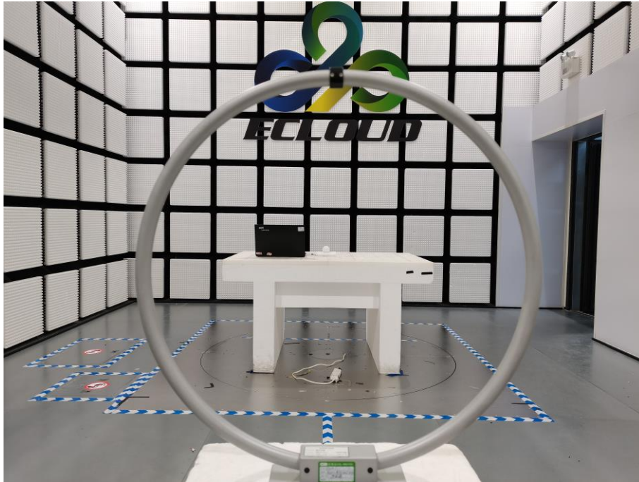
Fig. 1 Radiated emission setup photo(Below 30MHz)
