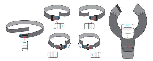
Once sensors are placed in the bands, put each band onto its corresponding body part (see image below). Connect hook and loop fasteners of shoulder band if desired. Make sure the elbow sensor is sitting behind the patient's elbow. Adjust bands for comfortable fit, if necessary. Log in on the tablet. Add new patient or select patient from directory; edit patient information as needed.
