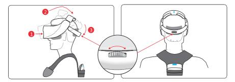
**Note:** Size of headset strap and interpupillary distance can be adjusted for fit. Top of head pad may be removed temporarily for better fit on larger heads.
