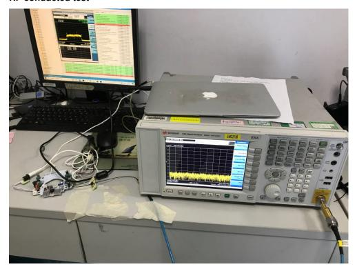
Conducted Emissions at AC Power Line (150kHz-30MHz)
