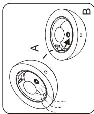
To avoid water entering the unit and damaging diffuser components, do not pour from the air outlet accessory side (see diagram B).
