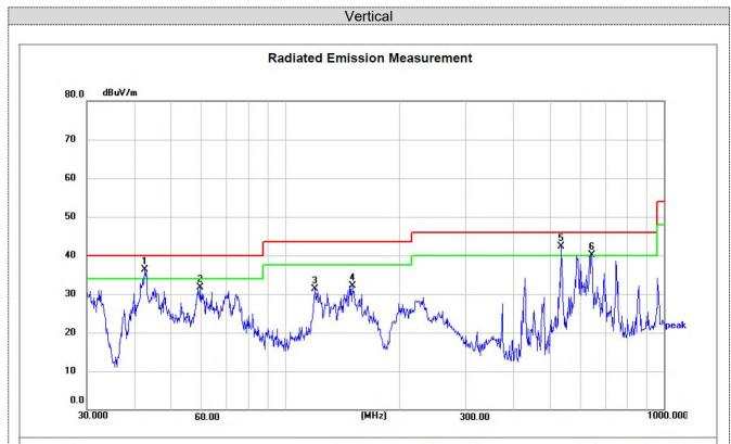
Site LAB Limit: FCC Part15 RE-Class B\_30-1000MHz
