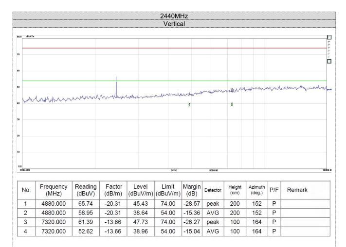
Note:1).Emission level (dBuV/m) =Raw Value (dBuV)+Correction Factor (dB/m)
