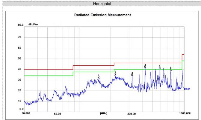
Site LAB Limit: FCC Part15 RE-Class B\_30-1000MHz
