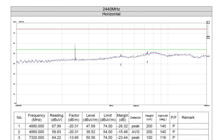
Note:1).Emission level (dBuV/m) =Raw Value (dBuV)+Correction Factor (dB/m)
