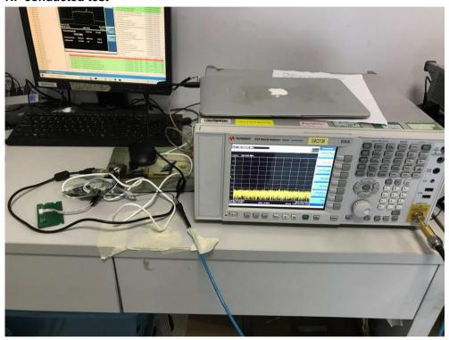
Conducted Emissions at AC Power Line (150kHz-30MHz)
