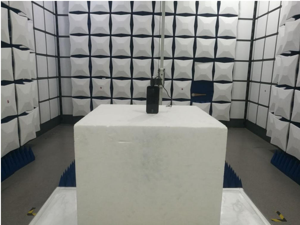
RADIATED EMISSION TEST SETUP ABOVE 1GHZ
