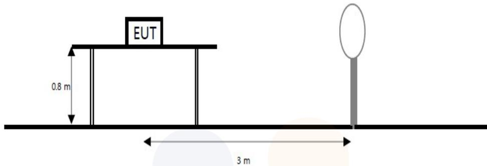
The diagram below shows the test setup that is utilized to make the measurements for emission from 30 MHz to 1 GHz emissions.
