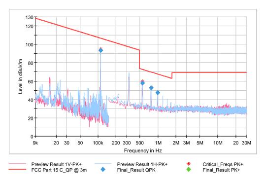
Test Mode - 5 V Charging Mode (Battery less than 50 % charged)
