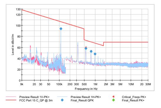
Test Mode - 5 V Charging Mode (Battery less than 100 % charged)
