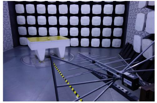
1.2 Radiated Emissions Test Setup
