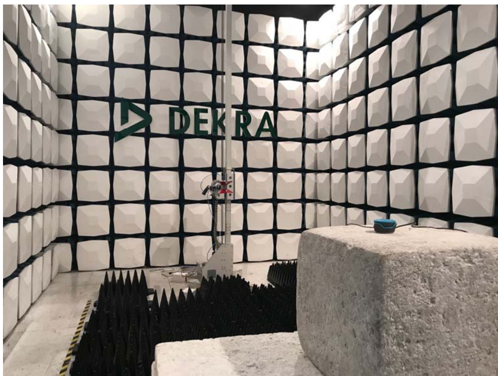
Description: Radiated Emission Test Setup for 1~18GHz
