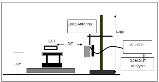
(B) Radiated Emission Test-Up Frequency 30MHz~1GHz
