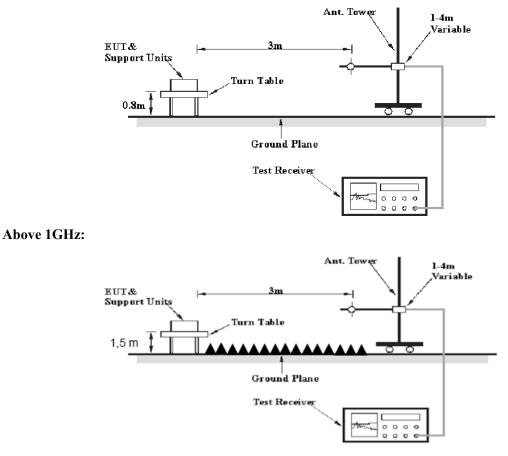
The radiated emissions were performed in the 3 meters distance, using the setup accordance with the ANSI C63.10-2013. The specification used was the FCC 15.209, and FCC 15.247, RSS-247, RSS-Gen limits.
