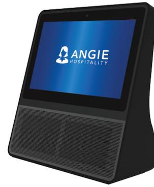
**1** Rapidly but lightly tap the logo at the top-center edge of the Spark's display seven times to reveal a drop down menu
